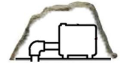
AERATOR IN DRY VENTILATED LOCATION
